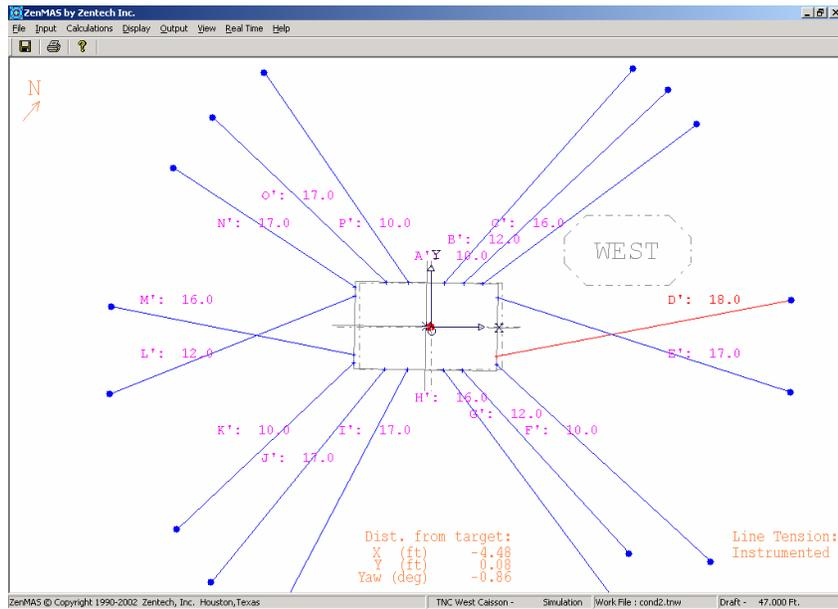
**Figure 2 Plan View Displaying Line Tensions**
