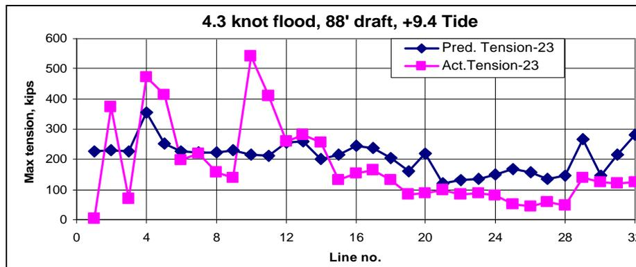
**Figure 5 Comparison of actual vs. predicted line tensions**
