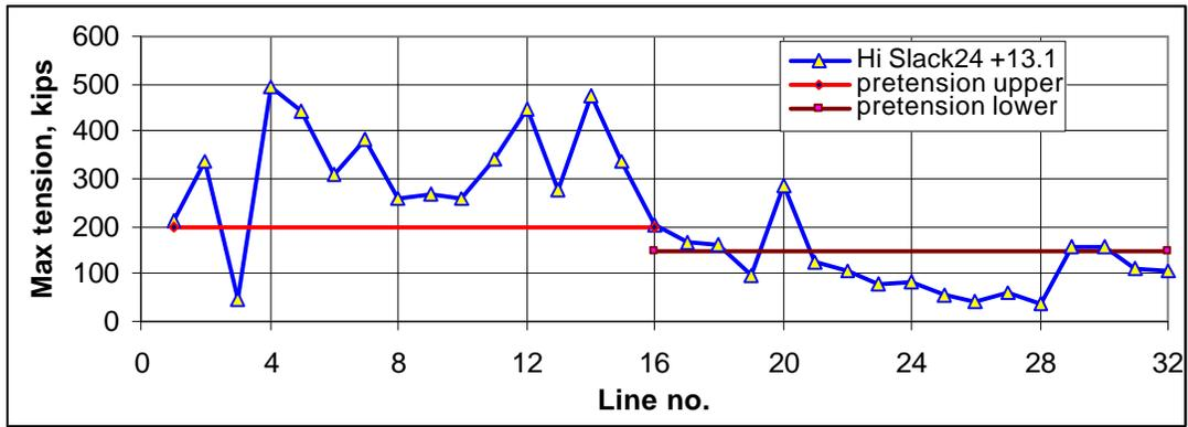
**Figure 10 Variation of Pretension between Lines**
