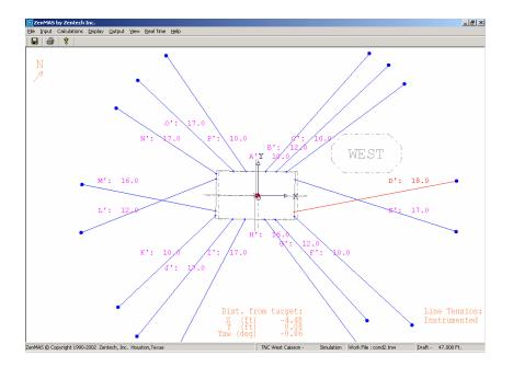
Figure 2 Plan View Displaying Line Tensions
