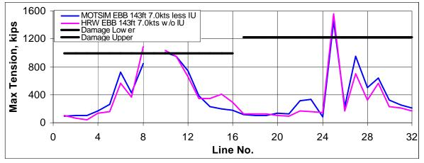
Figure 11 Comparison of Maximum Line Loads of HRW and MOTSIM Data 143 ft Draft 7 knot Ebb I upper removed – modified pretensions
