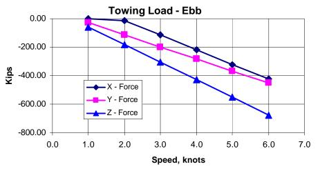
Figure 9 Towing Loads at 47-ft Caisson Draft
