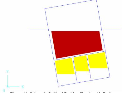
Figure 16 Caisson in Inclined Position Showing Air Pockets
