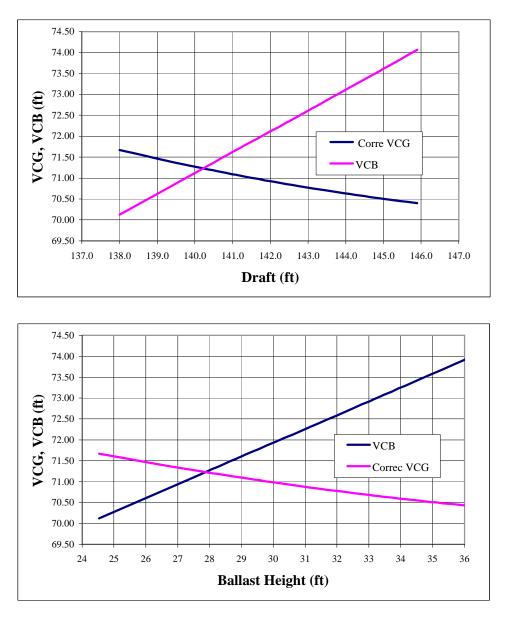
Figure 17 Plots of Corrected VCG and VCB
