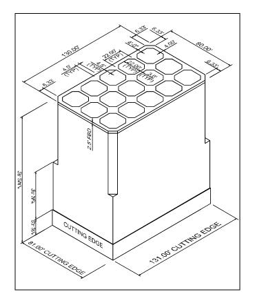
Figure 2 Caisson Geometry - Elevation
