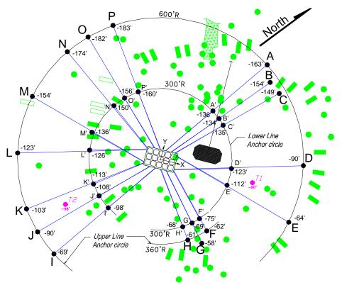
Figure 4 Anchor System Design Layout for the East Caisson
