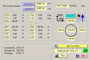
Part of Zentech's Suite of Load and Stability Calculator (LoStab) Programs, WMS is an interactive, menu-driven, vessel-specific software used in data management and loading calculations in the dayto-day operations of Spars.
