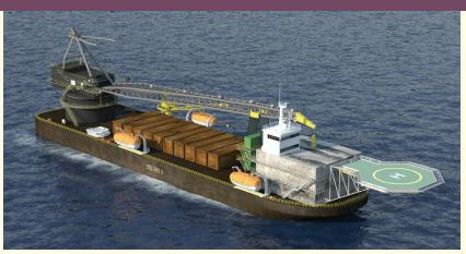
Zee Rig 3 shown with AmClyde Model 52 Marine Crane and 275 Ft. (83.8m) Boom.
