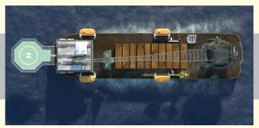
Plan view of Zee Rig 3 showing Main Crane and Utility Crane.
